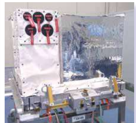
Figure 2: (below) The ASIM instrument mounted on CEPA. MXGS is on the right (silver cover), MMIA is on the left.
