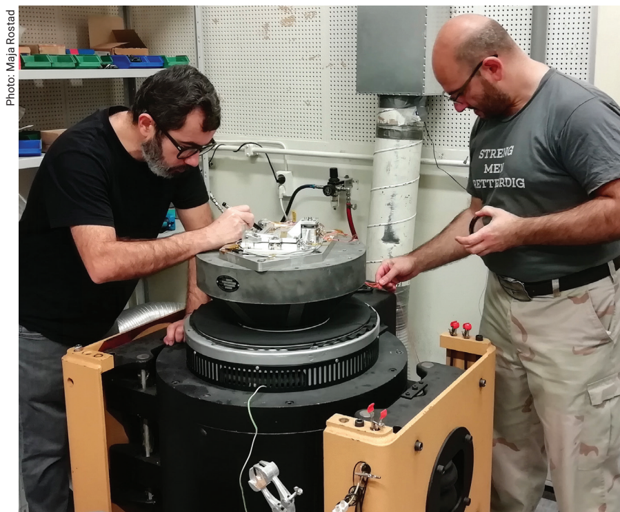
Figure 6: UiB engineers Nuno Roque (left) and Georgi Genov setting up the second bread board of the Radiation Shutter Bread Board (RSM BB2) on the vibration shaker at Prototech.
