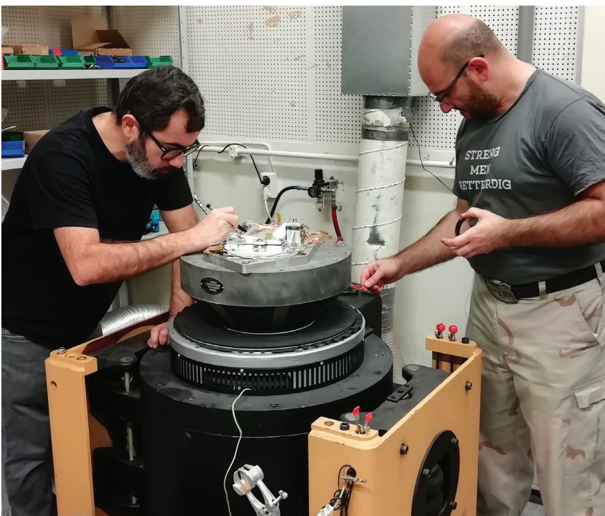
Figure 6: UiB engineers Nuno Roque (left) and Georgi Genov setting up the second bread board of the Radiation Shutter Bread Board (RSM BB2) on the vibration shaker at Prototech.
