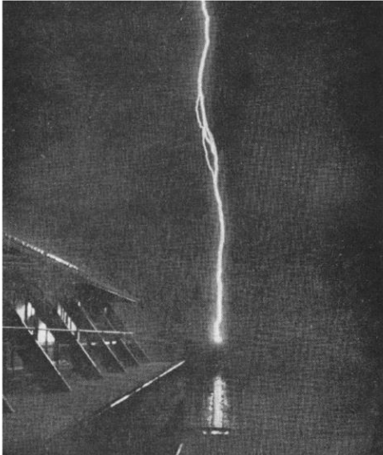
Fig. 4.28. A photograph of a lightning strike to a chimney pot showing a split in the channel, interpreted as evidence of an upward connecting leader. Adapted from Golde (1967).
