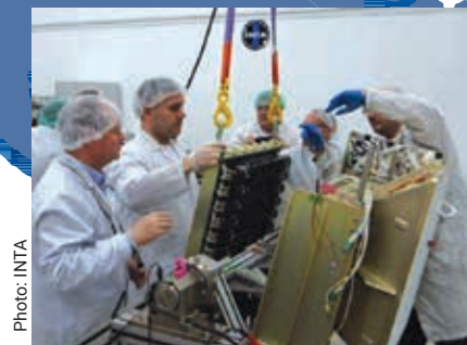
Figure 2: (Above) The HED is integrated into MXGS at INTA.
