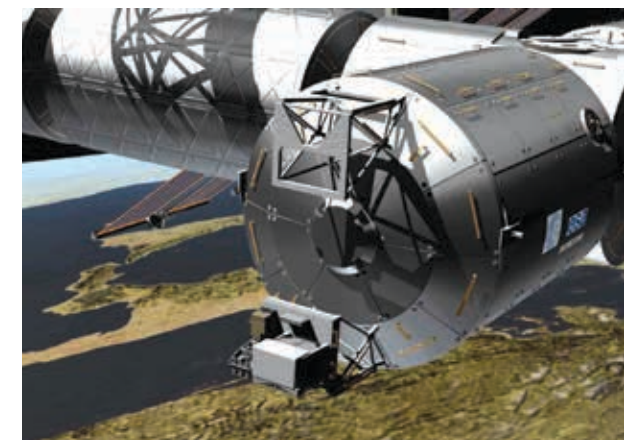
Figure 6: Above An illustration of the ASIM payload outside the Columbus module (lower left) Courtesy, Danish Technical University
