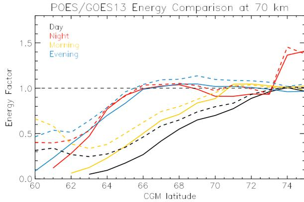
**Figure 4.** The estimated energy deposition ratio between the POES satellites (16–19) and METOP02 and GOES 13 for four MLT sectors at 60°–75° CGM latitude in the Northern Hemisphere. The solid lines are based on the vertical detector and the dashed lines are based on the horizontal detector.
